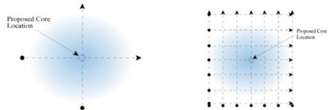
For detailed feature mapping in smaller areas with little known information, 3-D scanning is often utilized. A 3-D investigation compiles multiple parallel and perpendicular 2-D lines into a panel or panels. Performing 2-D scanning
