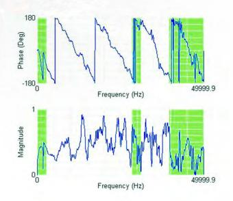
The plot above shows a phase plot and coherence plot that have been masked for data collected on the top of a concrete drilled shaft. The masked out areas are unwanted boundary reflections from the round shape of the drilled shaft.
