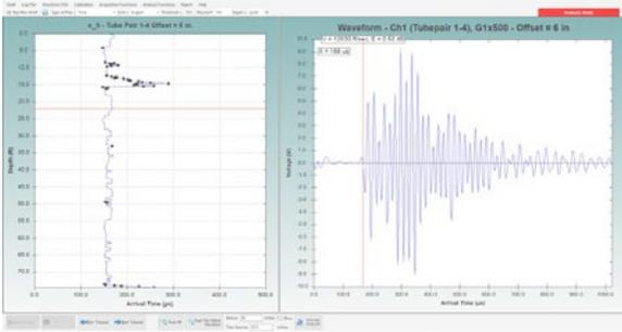
*New WINCSL software tomogram example, 6 inch offset, 2 defects visible at 15 feet plus the bottom*
