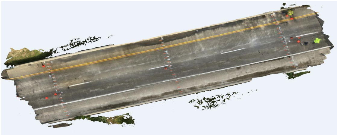
Figure 13. Digital orthomosaic (photogrammetric image) of concrete bridge deck
