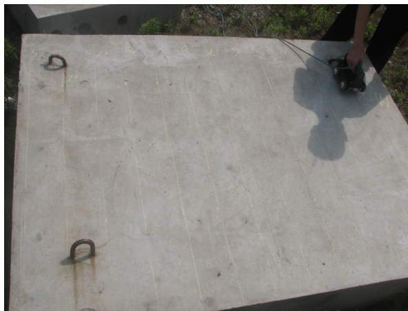
Figure 2 – Impact-Echo Test Using an Impact-Echo Scanner on a Mock-up Panel
