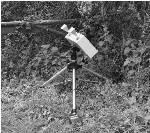
Figure 6. View of the new IBIS-S sensor
