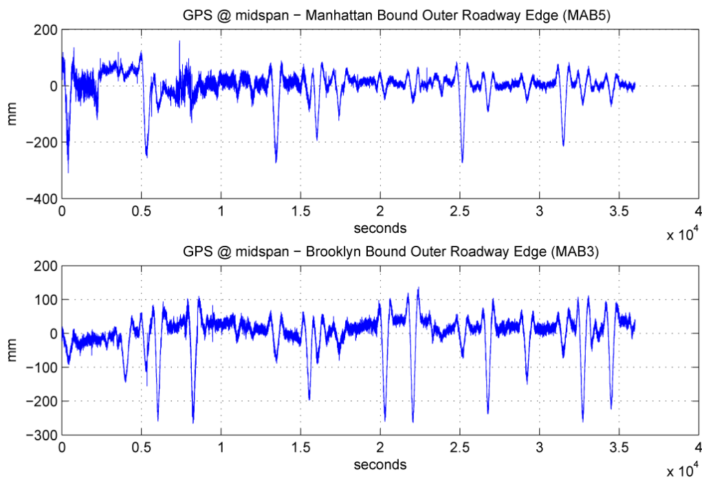
Figure 5. GPS receiver data showing the outer roadway edge deflections of the Manhattan Bridge
