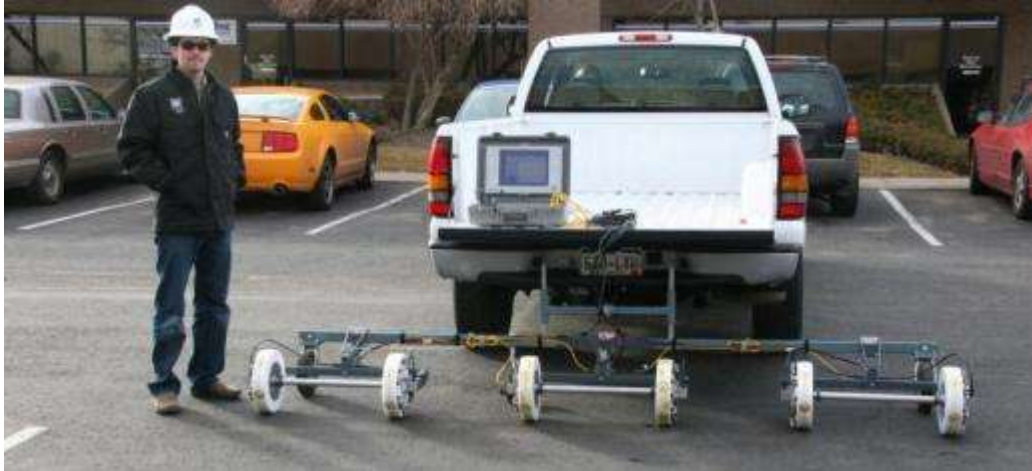
Figure 2 – Bridge Deck Scanner Towed behind a Vehicle – 3 pairs of wheels at 2 feet (0.61 meter) apart
