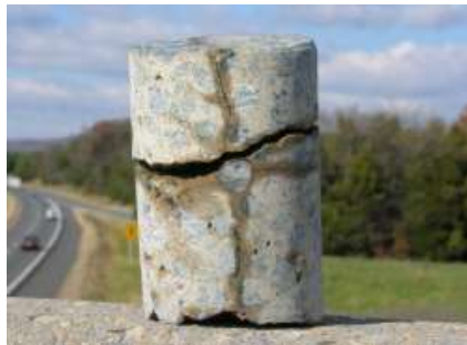
Core # 5 - Delamination Depth at 2.5 inches
