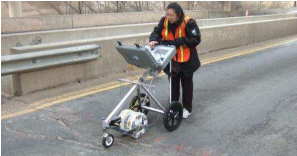
Figure 3 – BDS System Attached to a Scanning Cart on Asphalt Overlaid Deck – Single Pair of Wheels at 6 inches apart for Combined Impact Echo/Surface Waves Scanning
