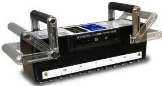
(c) UST inspection using A1040 MIRA ultrasonic tomograph
