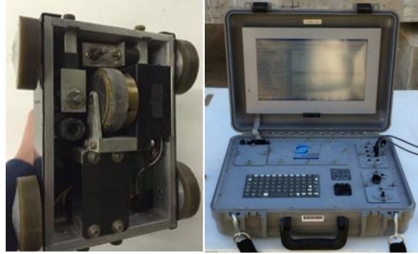
(b) IE scanner and DAQ PC
