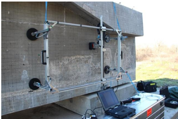
(d) USE inspection with dual element probe mounted on an automated scanner
